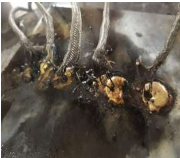
Fig 2: Thermocouple wires connected to the specimen.
