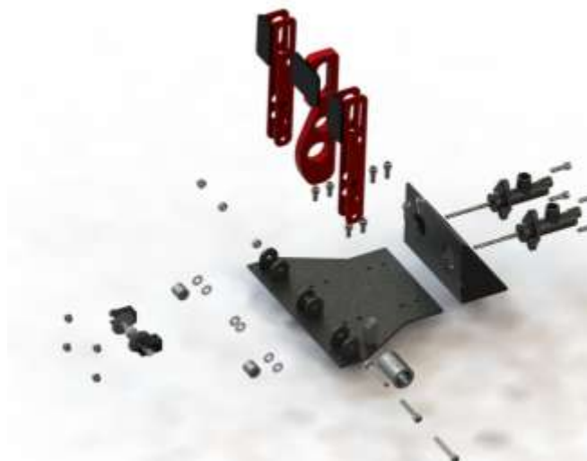
Fig -23: Pedal assembly exploded view
