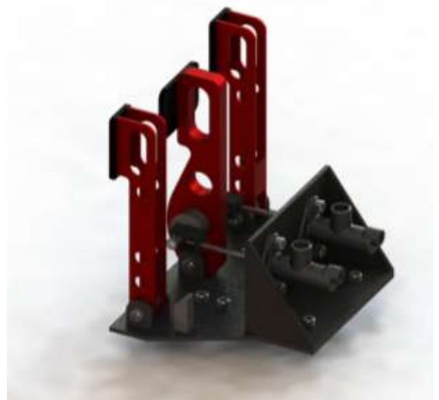
Fig -22: Pedal Final Assembly CAD model
