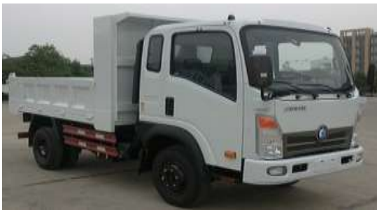
Fig 3.3: A dump tipper with dump box dimension- 3000 x 1820 x 600mm (source: https://www.alibaba.com/product-detail/Sinotruk-CDW-Dongfeng-Foton-Brand-Light_60444959145.html?spm=a2700.7724857.normalList.15.29ed5a12DP0ytb )
