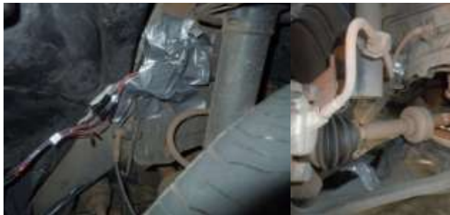
Fig 2: Accelerometer positioned on the sprung mass (left) and accelerometer positioned on the unsprung mass (right).
