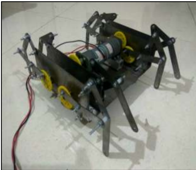
Picture 1: The prototype of the octopod spider robot
