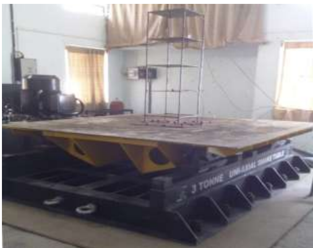
Fig-2: Model Fixed On Shake Table
