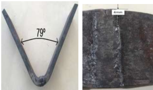
Fig 13: Bend test sample 5 (PWHT at 640°C)
