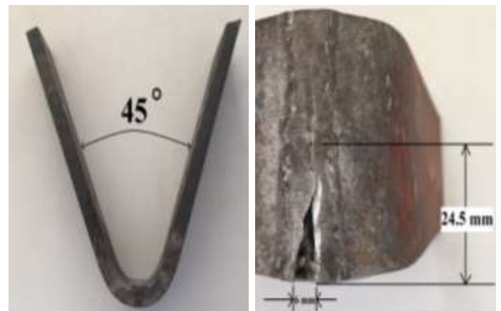
Fig 12: Bend test sample 4 (PWHT at 610°C) Sample 5: PWHT at 640°C
