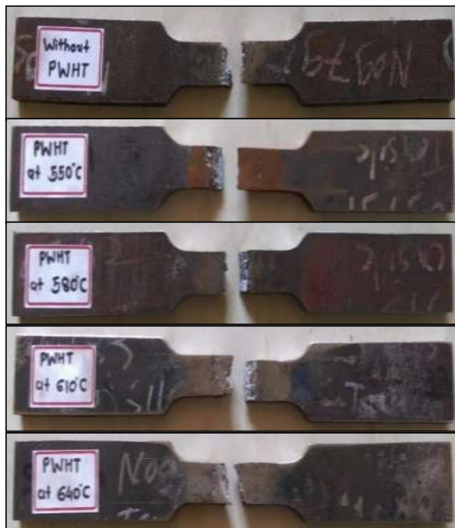
Fig -5: PWHT Test
