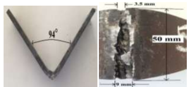
Fig 10: Bend test sample 2 (PWHT at 550°C) Sample 3: PWHT at 580°C
