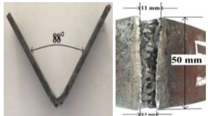
Fig 11: Bend test sample 3 (PWHT at 580°C) Sample 4: PWHT at 610°C
