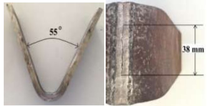
Fig 9: Bend test sample 1 (Without PWHT) Sample 2: PWHT at 550°C
