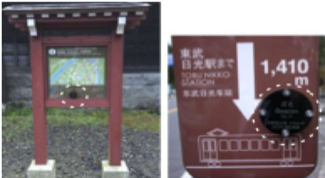
Fig -2: BLE Beacon on the road (in dotted circle)
