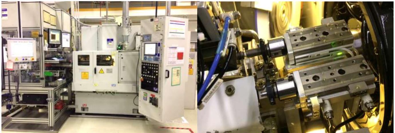
Fig 11: On the left: Handling system and grinding machine. On the right: Gripper mechanism
