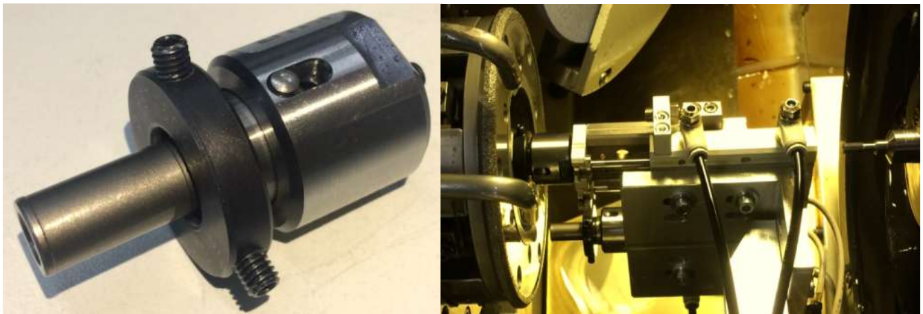
Fig 12: On the left: Gripper and workpiece. On the right: Unload from chuck when the pneumatic piston is extended
