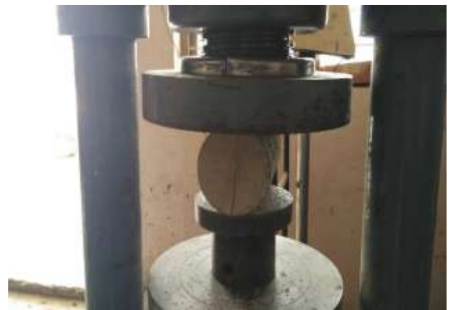
Fig. 3.3: Split tensile test on cylinder
