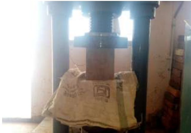
Fig 3.1: Compression test on cube
