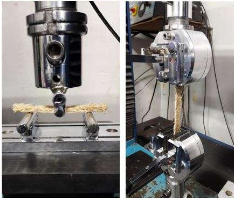
Fig 2: Tests, Flexural (Left), Tensile (Right)
