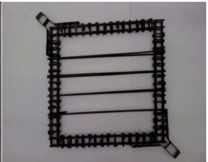
Fig-2: Reinforcement details of specimen
