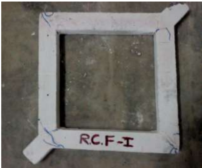
Fig-5: Failure pattern of RC frame without infill
