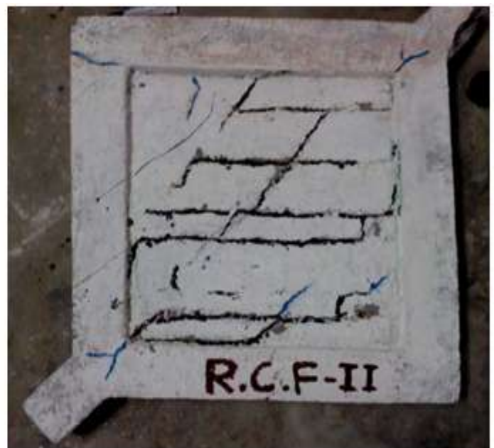
Fig-7: Failure pattern of RC frame with infill
