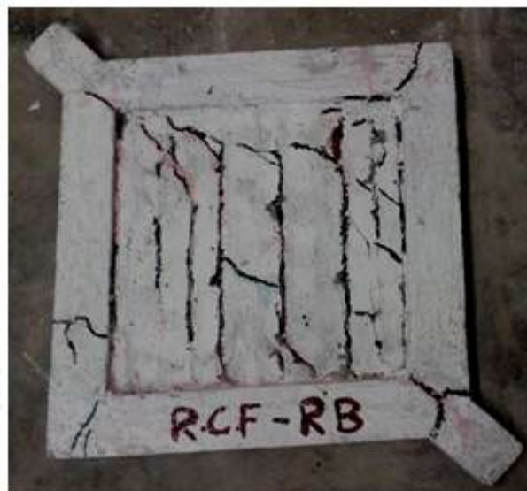
Fig-9: Failure pattern of frame with connector
