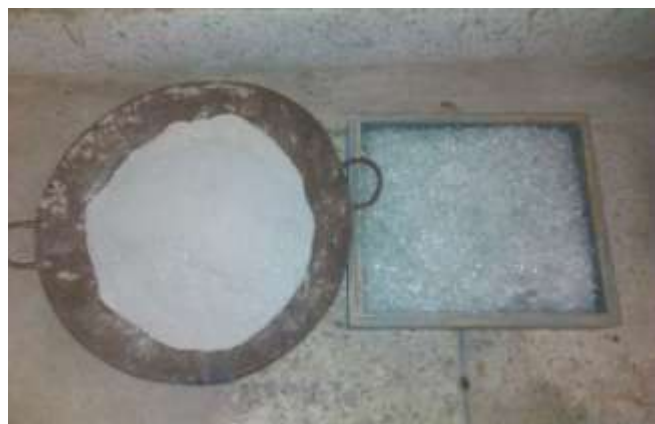
Fig -1: Crushed waste glass
