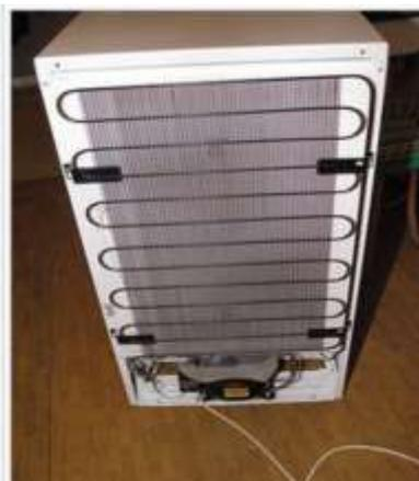
**Fig 1:** Condenser of refrigerator
