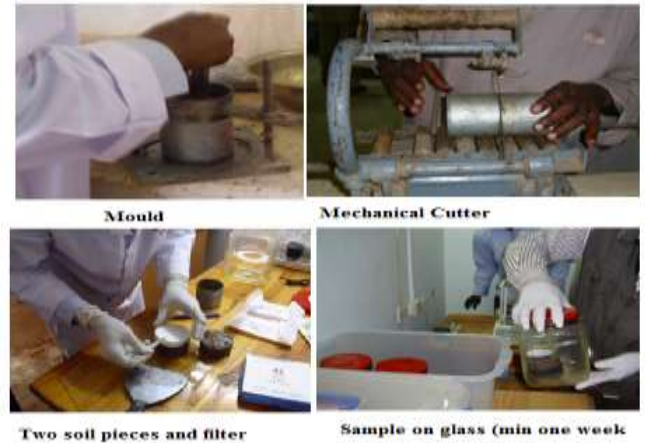
Fig -4: Soil suction procedure
