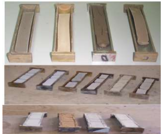
Fig -1: Final length of LS for different samples after oven drying
