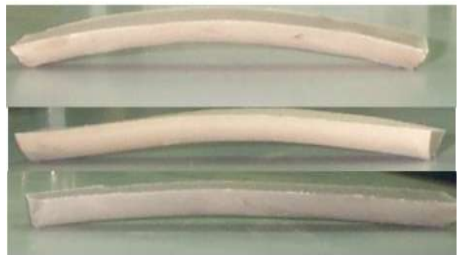
Fig -2: The hogging phenomenon for some soil samples
