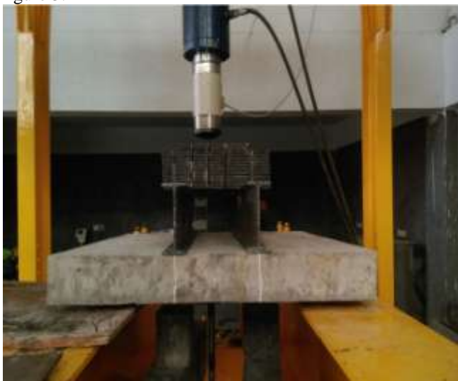
Fig 3: Experimental setup for flexural test
