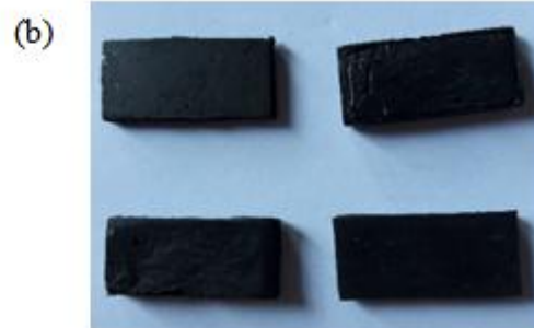
Fig 2. (a) Microwave rubber based absorber filled with \text{SrFe}_{12}\text{O}_{19} particles (b) Fabricated sample filled with \text{SrFe}_{12}\text{O}_{19} particles
