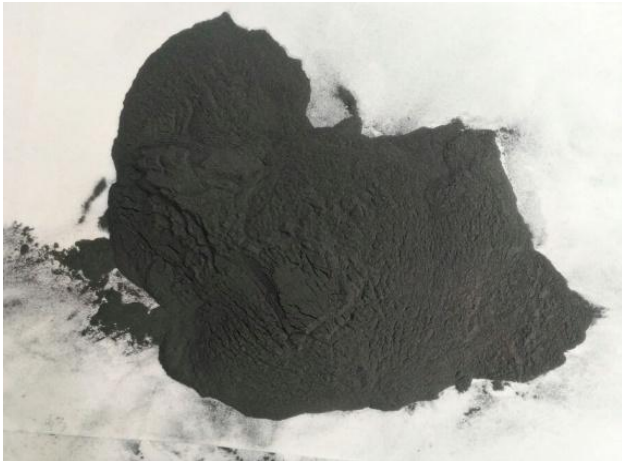
Fig-1.3: Preheated Silicon Carbide particles
