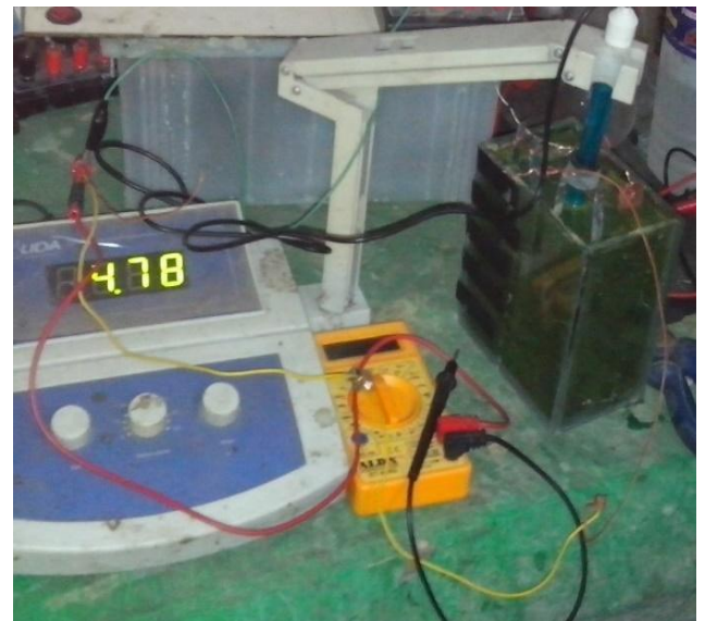
Fig -2: An experimental set-up of studying the self-discharge characteristics of BPL cell [8].
