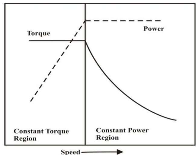
Fig-5: Ideal mechanical characteristics of electric motor in EV
