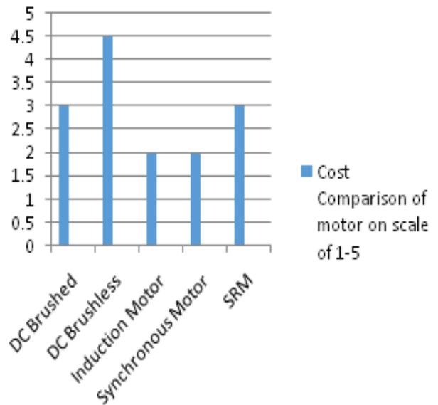
**Chart -3:** Cost of motor Comparison for Different Electric Motor
