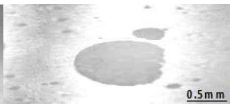
Fig-2: Actual shrinkage and pores defects of steering servo shell
