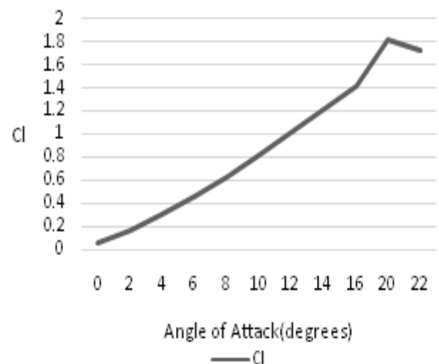
Chart -2: Variation of coefficient of lift with angle of attack
