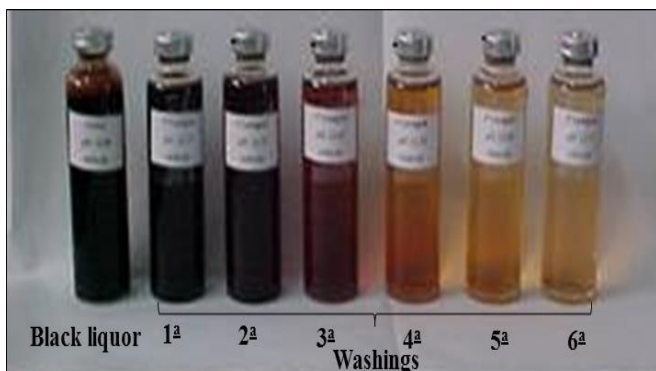
Fig 3 – Effluent samples from the stage of cotton pulping, with emphasis on the color difference of washing water effluents [5]
