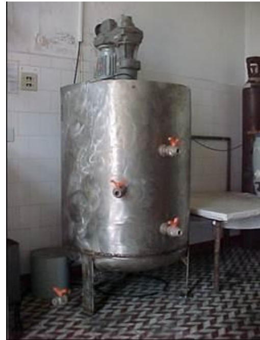
Fig 2- Biological reactor / 500L capacity
