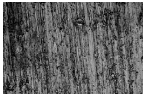
Fig 19: Scanned electron micrograph of wear surface of sample 5
