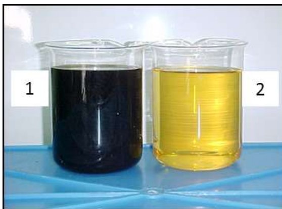
Fig 4 - Effluent: 1) before treatment and 2) after chemical treatment
