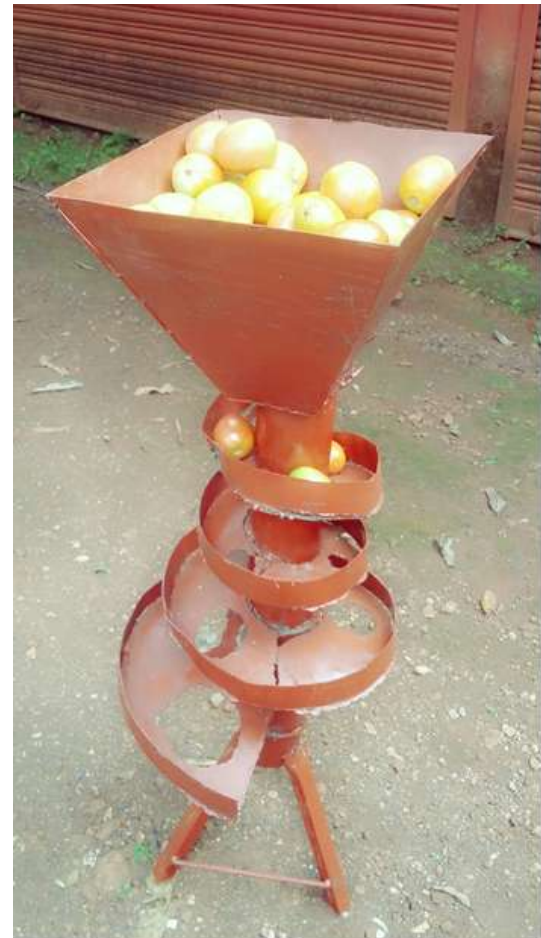
Fig-2: Sorting of tomatoes with the help of gravity type fruit sorter
