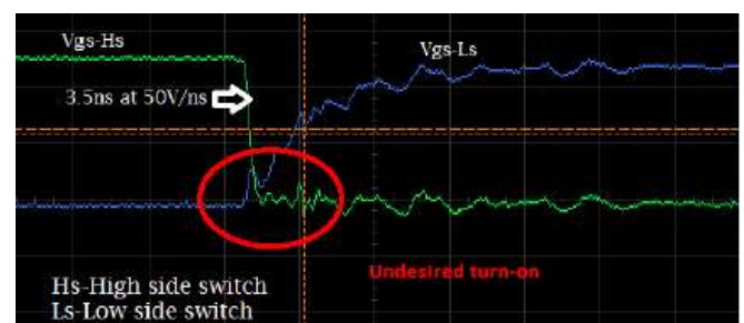
Fig 3: Shorting of the leg due to cross-conduction
