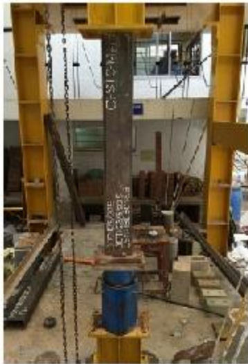
Fig 6: Test setup for testing of CFST columns of 1m and 1.5m.
