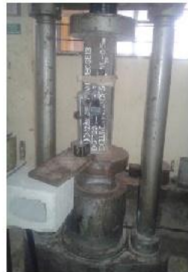
Fig 5: Test setup for testing of CFST columns of 0.5m height in CTM.
