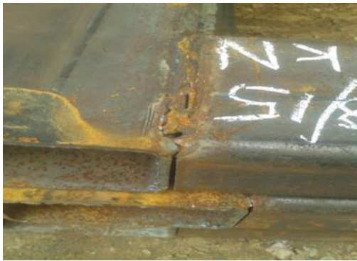
Fig 10: Connection failure of the specimen HSTF-01.
