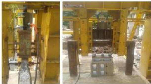
Fig 7: Test set up for the testing of CFST frames.
