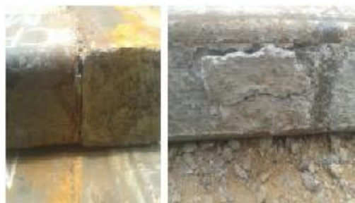
Fig 11: Concrete crushing in the beam portion of CFST frame.
