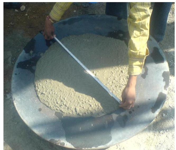
Figure – 2: Flow test
