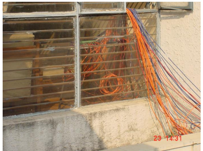
Figure 14 : Instrumentation Wires embeded in UHPFRC and Conventional Pavement in front of the Canteen by Staff of Bridges Div.)
