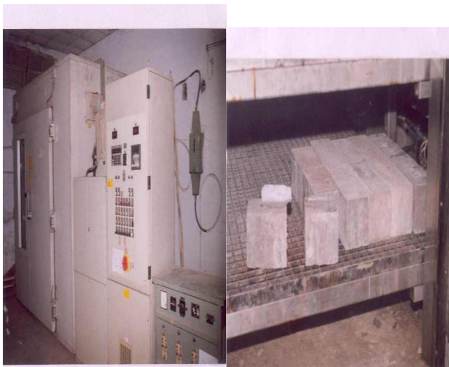
Figure 11 ; Durability Weathering Chamber at CRRI for Durability test.
