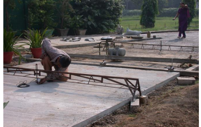
Figure 12: Evaluation (Deflection) of UTWT Using Dial Gauges at CRRI Curling of UTWT was found maximum 0.2 mm)
