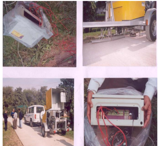
Figure 13 Evaluation of UHPFRC Using Instrumentation (FWD and Temperature Sensors)
