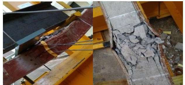
Plate 14: Crushing of concrete at mid span
