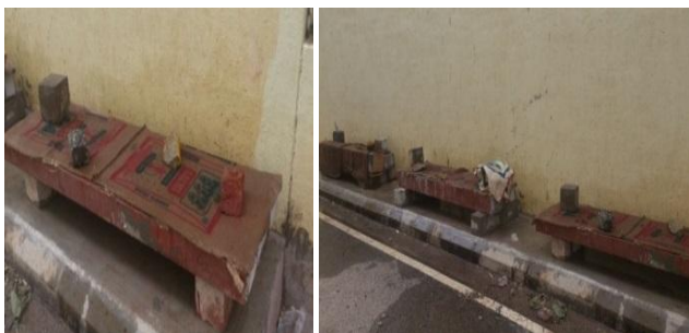
Plate 9: Beams are covered with gunny bags and cured for 28 days
