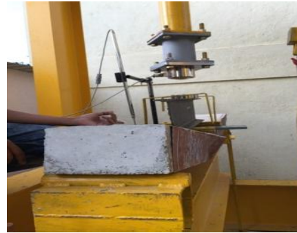
Plate 13: Slip of concrete at the ends
