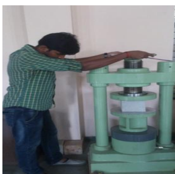
Plate 10: Cubes tested in compressive testing machine for 28 days strength.
