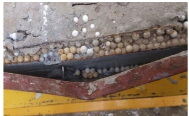
Plate 15a: Protrude of shear connectors from the concrete in light weight concrete infilled beams
