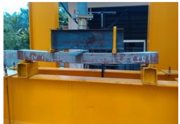
Plate 11: Arrangements of specimen on the loading frame.
