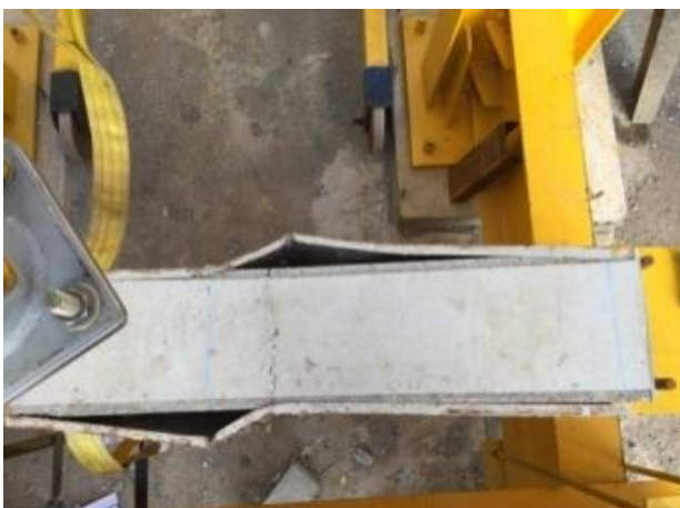
Plate 12b: Buckling of steel in compression zone in normal concrete infilled beam.
