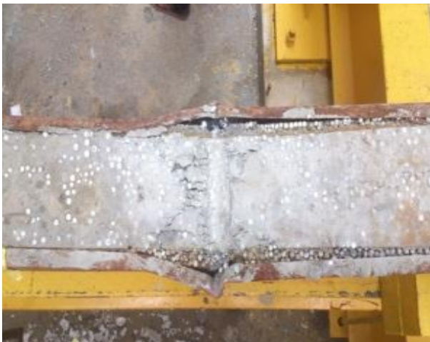
Plate 12a: Buckling of steel in compression zone in light weight concrete infilled beam.
