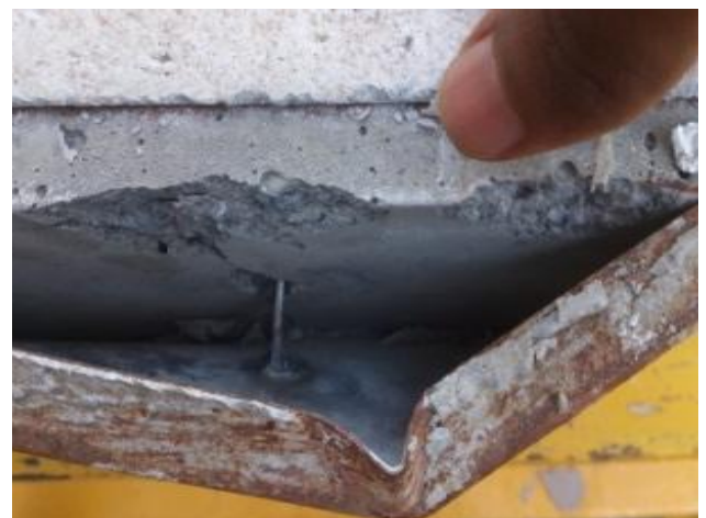
Plate 15b: Protrude of shear connectors from the concrete in normal concrete infilled beams
