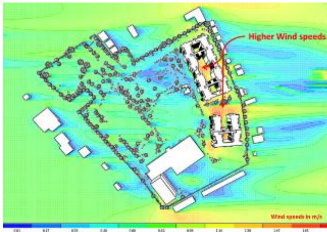
Fig 2 Outdoor wind flow pattern (horizontally) at site plan level
