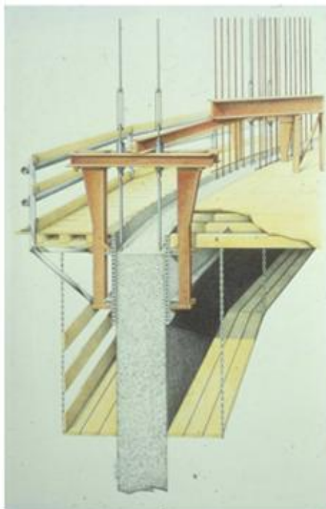
Fig -1: Slip Form assembly
