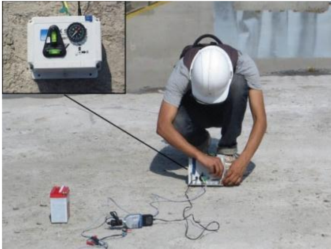
Fig - 4: Leveling and Aligning of sensor on roof top
