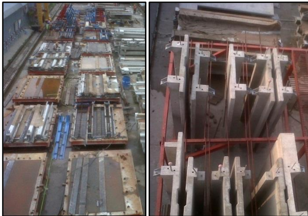
Fig -5: Casting /Stacking at Yard
