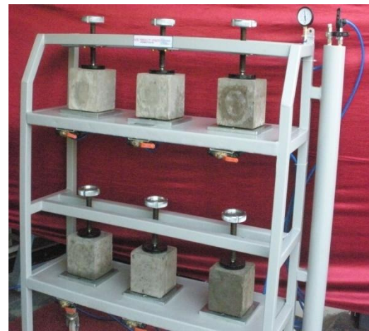
Water permeability test system as per DIN -1048
