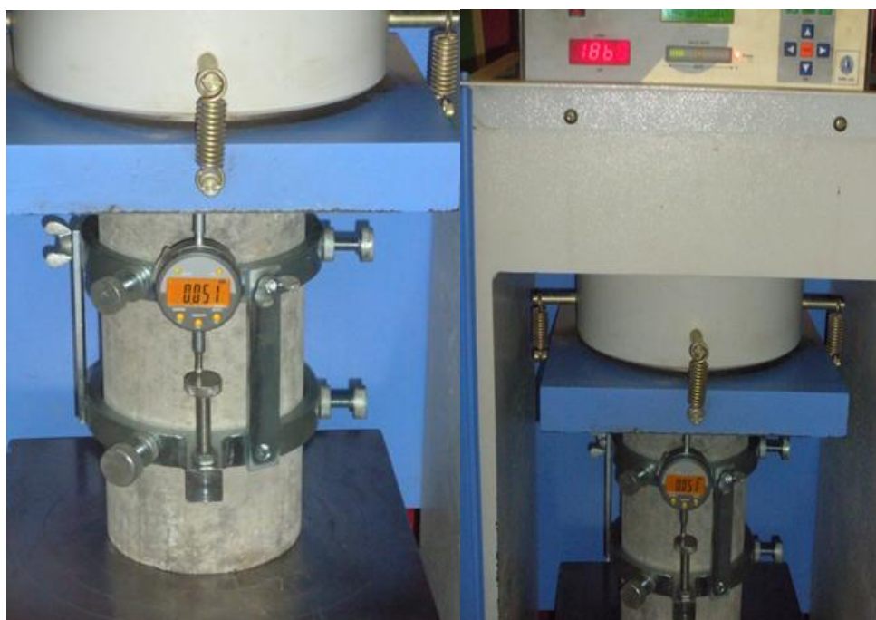
Modulus of Elasticity ['E'-Value] as per ASTM-C-469-02 under process
