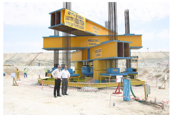
Figure 7. Pile load test of Burj Khalifa.
