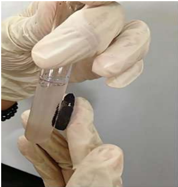
Fig 1: A suspension of MIONs getting attracted to a permanent magnet
