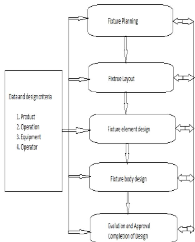
**Fig 1** various aspects of fixture design
