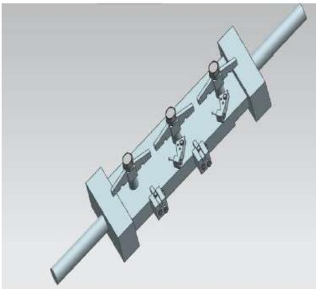
**Fig 3.** 3D View of Fixture Assembly
