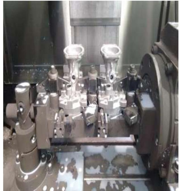
**Fig 4** Fabricated Fixture is used in machine for Manufacturing
