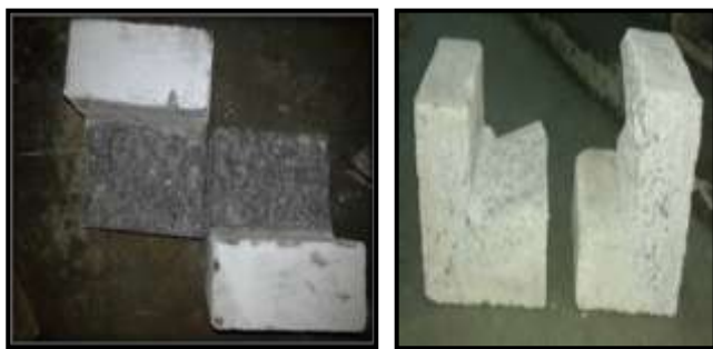
Fig 6: Failure pattern in NSC Fig 7: Failure pattern in GPC
