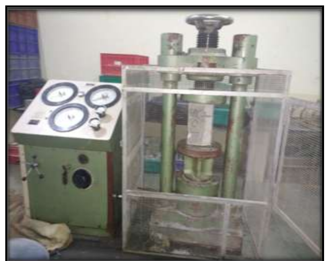
Fig 4: In-plane shear strength test arrangement under CTM
