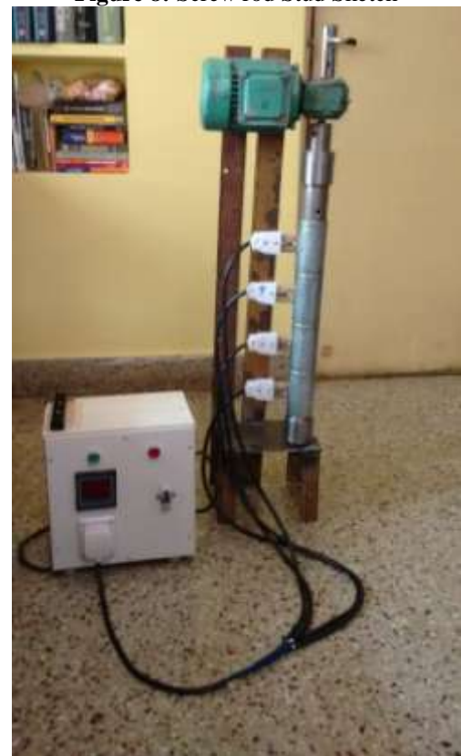
Figure 9: A photograph of the completed Screw extruder
