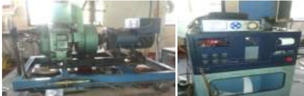
Fig.2 Diesel Engine Test Rig with AVL 444 DI gas analyzer and AVL 415 smoke meter
