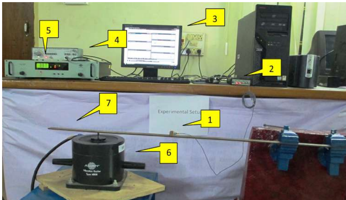
Figure 1: Experimental Setup 1. Vibration Pick-up, 2. Vibration analyzer, 3. Vibration indicator, 4. Function generator, 5. Power amplifier, 6. Vibration Exciter, 7. Cantilever beam specimen.
