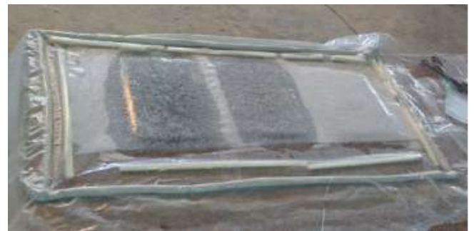
Fig.3. shows the vacuum molding process carried out.
