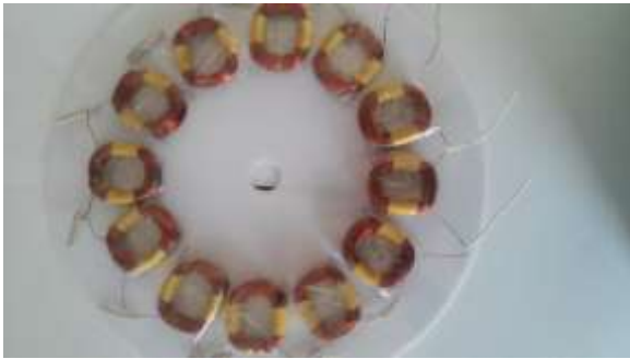
Fig 5 Copper Windings of the AC Turbine
