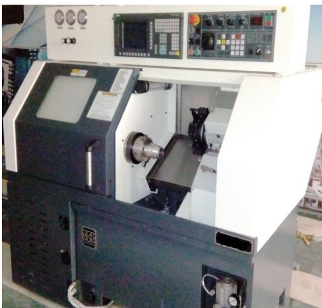
Fig 2. ACE Micromatic Apollo CNC Turning Machine
