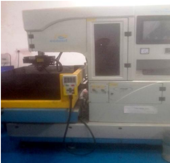
Fig 1 Setup of ECOCUT CNC Pulse Generator ELPULS-15
