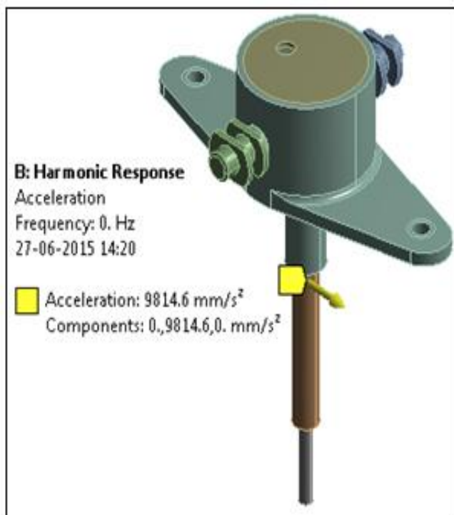
Fig 6 Acceleration load is applied to T50 thermocouple in Y-direction
