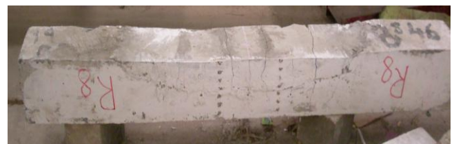
Fig 8. R_5 (EMACO S46C T) failed in flexural crack
