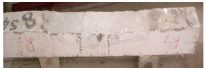
Fig 7. R_4 (EMACO S48C T) failed in flexural crack
