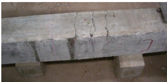
Fig 3. Control beam (C) failed in flexural crack
