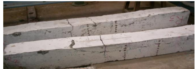
Fig 6: R_2 beam (FA mort) failed due to debonding and R_3 beam ((SF+FA) mort) failed in flexural crack
