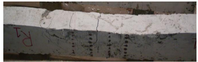
Fig 5: R_1 beam (SF mort) failed due to debonding
