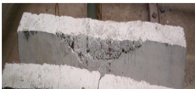
Fig 4. R_{NC} beam (repaired with normal concrete) failed in flexural crack
