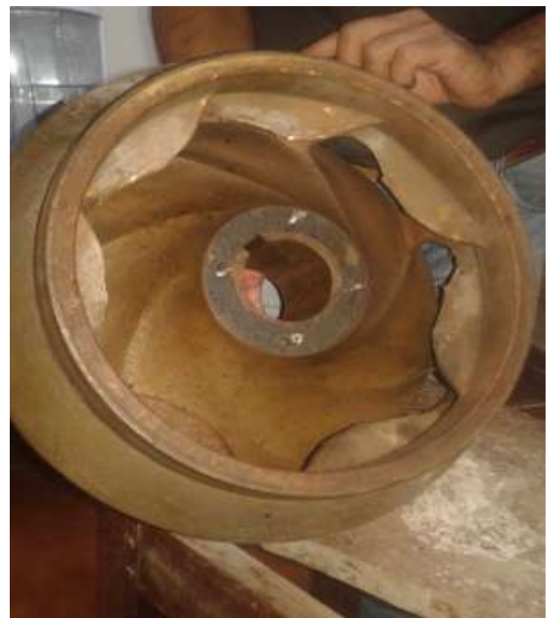
Fig -2: Worthington 5 Hp Vertical turbine impeller (Dapora, Jalgaon water supply station)
